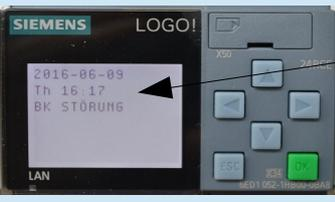
The image shows the same Siemens LOGO! control panel. The display now shows the date '2016-06-09', the time 'Th 16:17', and the status 'BK STÖRUNG'. A black arrow points from the text to the display.
