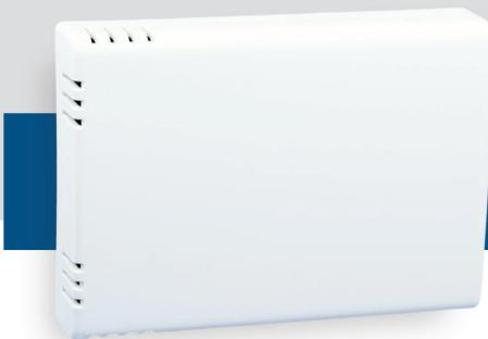
The RSH series are room sensors which measure the relative humidity in the air. Four pre-defined ranges provide ideal measurement windows with one user-definable range. The implemented digital sensor is self-calibrating and maintenance-free. These sensors are equipped with Modbus RTU (RS485) communication and have an analog output.
